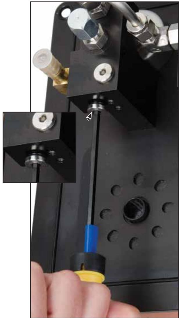
Use \frac{5}{32} " hex driver to remove plug.
